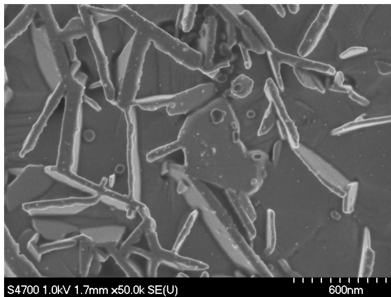
Figure III-50 FESEM Micrograph of Sample 20/1000/RA
