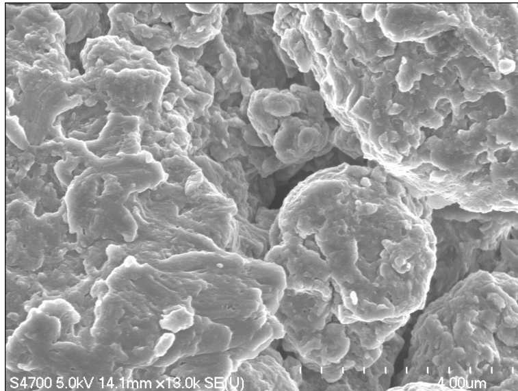
Figure III-31 Surface Smeared Particles Showing Flow Lines in As-milled RMM10h9TiAr Powder Particle 19kX
